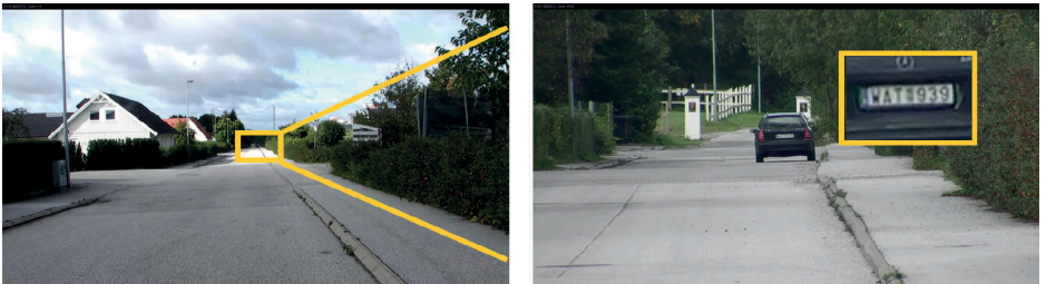
Figure 2.4p Wide view (left) and zoomed view (right) in an HDTV 1080p PTZ camera, allowing the license plate to be read at 275 m (900 ft.).
