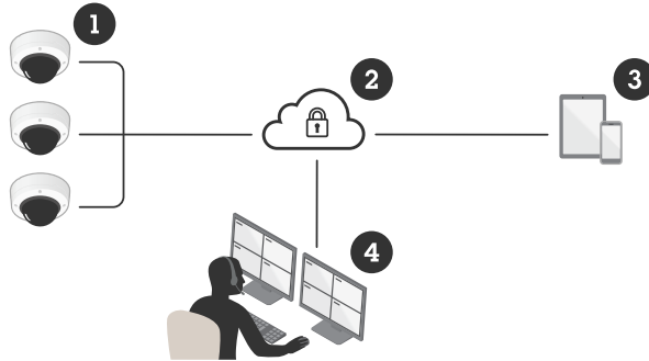
Figure 17.4b Overview of a hosted video solution. Video from the customer's site (1) is stored and managed in the cloud (2) by an alarm company. Live and recorded video can be accessed by authorized users through a computer or mobile device (3), and the alarm company can monitor the video remotely (4).
