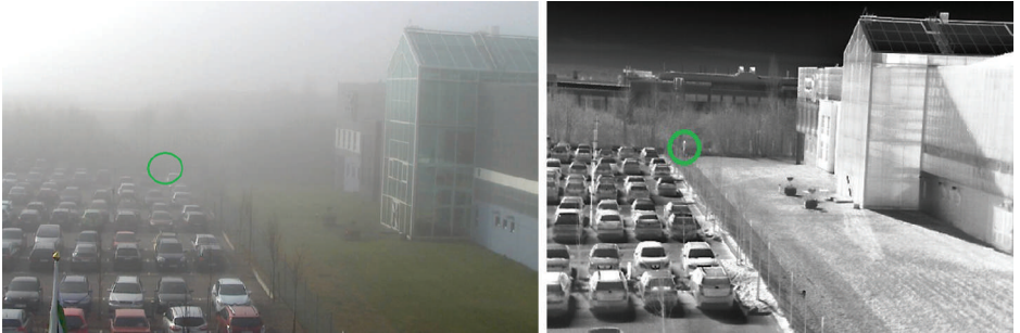
Figure 2.2d Left: image from a conventional camera on a foggy scene. Right: image from a thermal camera on the same foggy scene.
