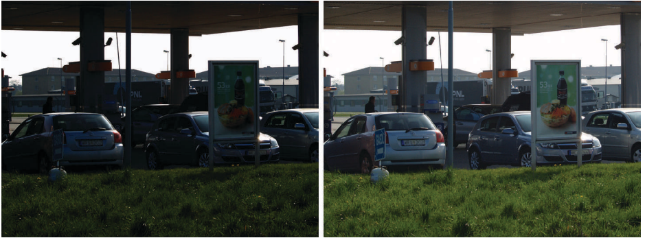
Figure 3.5a Strong backlight, without backlight compensation (left). With backlight compensation applied, the foreground is more visible (right).
