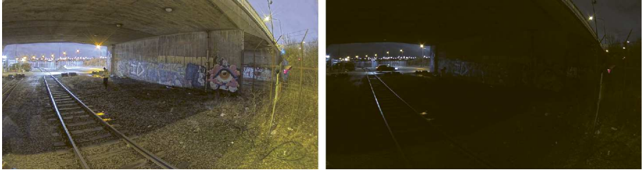
Figure 2.2a Left: a sharp, bright color image delivered by a Lightfinder 2.0 camera, even though the light intensity was only 0.05 lux under the bridge. Right: a snapshot of the same scene manipulated to visualize how the scene appeared to the human eye.
