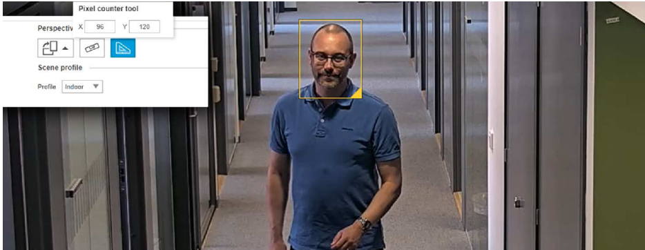
Figure 2.3b Axis pixel counter showing the pixel resolution of a face.
