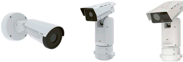
Figure 2.4t Thermal cameras in bullet (left) and fixed box mounted on positioning unit (center) form factors. The bispectral PTZ camera (right) combines a visual and a thermal camera in one unit for mission-critical surveillance.
