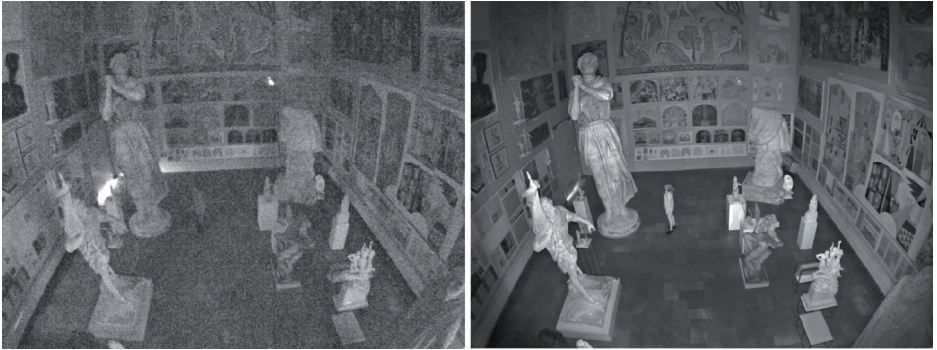
Figure 2.2c Left: night mode snapshot captured without illuminators (a small amount of light was admitted under a door in the left-hand corner of the room). Right: night mode snapshot captured using IR illuminators.
