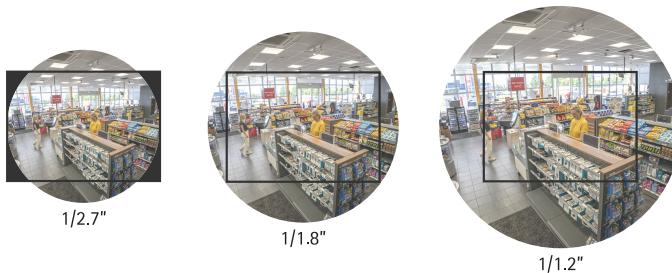
Figure 3.2h The effect of different lenses on a 1/1.8" sensor. Right: a 1/2.7" lens is too small for the sensor and the image has black corners. Center: a 1/1.8" lens matches the sensor size. Left: a 1/1.2" lens is too large for the sensor and the information outside the image sensor will be lost.
