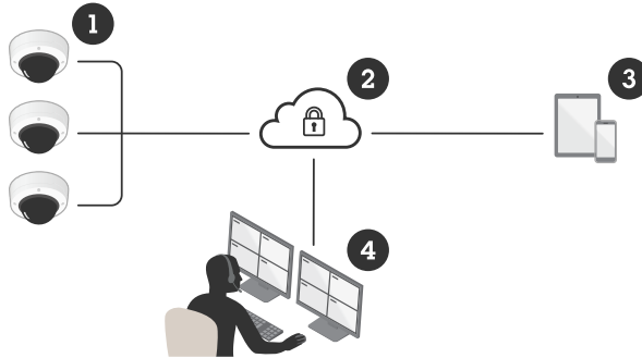
Figure 16.1c Overview of a hosted video solution. Video from the customer's site (1) is stored and managed in the cloud (2) by an alarm company. Live and recorded video can be accessed by authorized users through a computer or mobile device (3), and the alarm company can monitor the video remotely (4).
