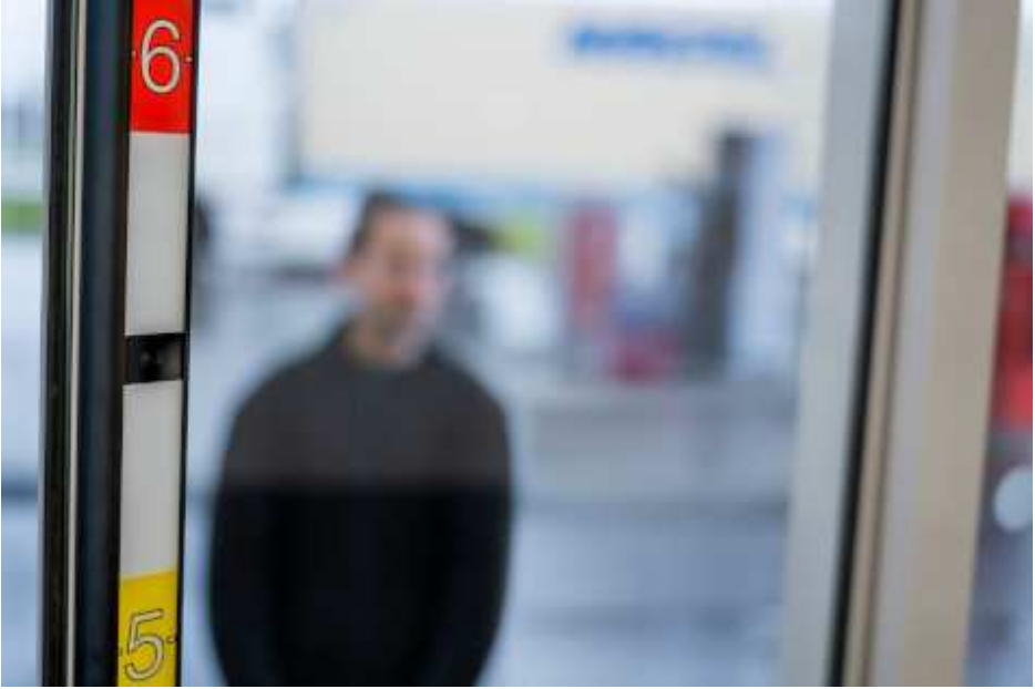
Figure 2.4m Designed to be placed near building exits, a height strip housing enables extremely discreet installation of pinhole sensors. The camera is positioned to look straight at a person's face for more reliable identification.
