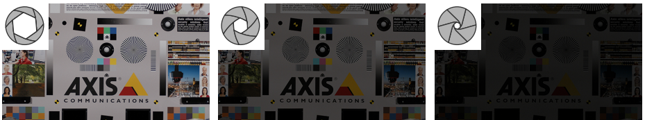
Figure 3.2d The light gathering ability of a camera is higher when the f-number is lower.
