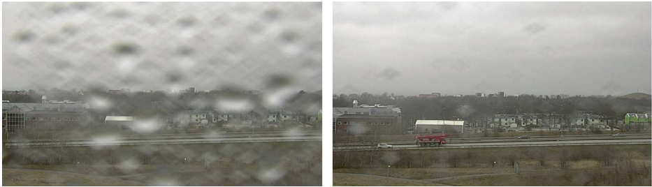
Figure 2.4s Two snapshots of the same rainy scene, before shaking (left) and after shaking off the water (right) using speed dry.
