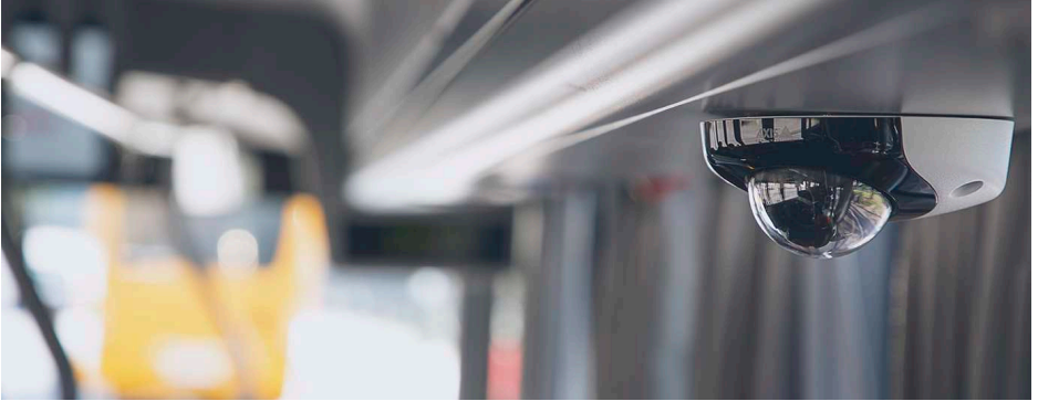
Figure 2.4e An onboard dome camera mounted in the ceiling of a bus.
