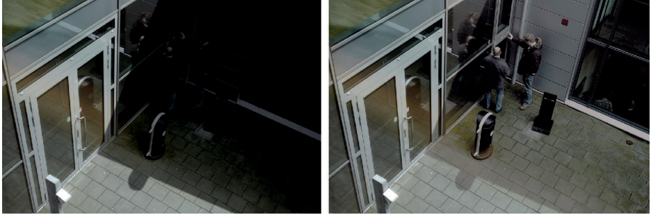
Figure 3.5b Two images of the same scene. The image on the right handles the dynamic range in the scene better, and details in both the bright and dark areas are visible.
