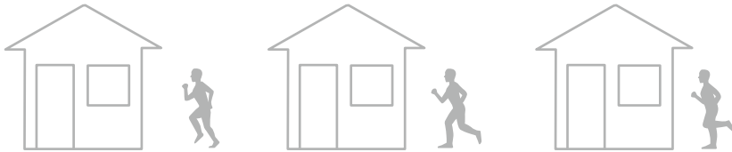
Figure 6.1a In the Motion JPEG format, the three images in the above sequence are coded and sent as separate unique images, with no dependencies on each other.
