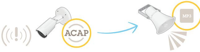
Figure 7.2a Unmonitored solution: a camera detects motion in a restricted area and sends a command to a speaker to play a prerecorded audio message.
