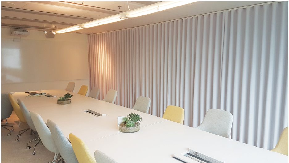
Figure 3.3a Curtains and other pieces of fabric can significantly improve room acoustics.
