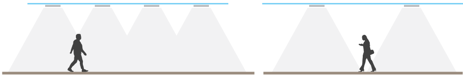
Figure 10.3a Left: in a premium solution, sound is even throughout the area. Right: in a basic solution, sound is less even, and spots with lower sound volume are allowed.
